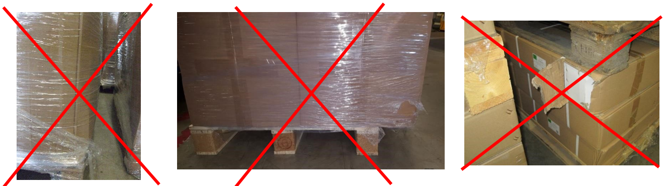
Figure 4: Not accepted – bulging / bursting and general protrusions
